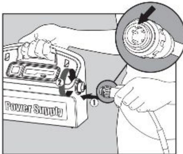
Plug in the power supply and leave it in the OFF position.
